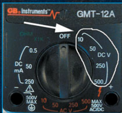
2. There are four typical functions found on almost all multimeters. The most common is DC volts.
